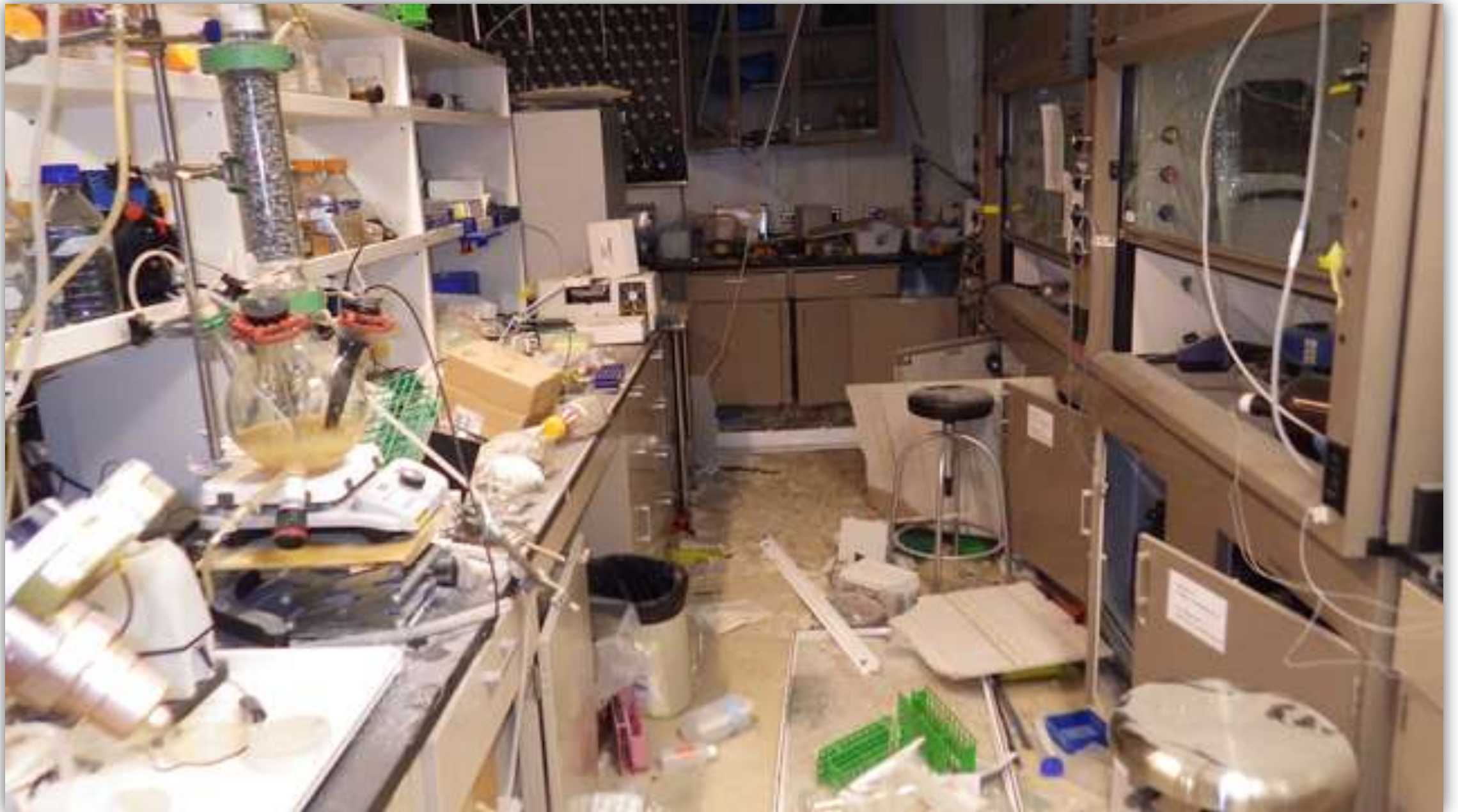
A powerful explosion at a University of Hawaii science lab was likely caused by a digital pressure gauge that shouldn't have been used around flammable gases (18/04/2016).
