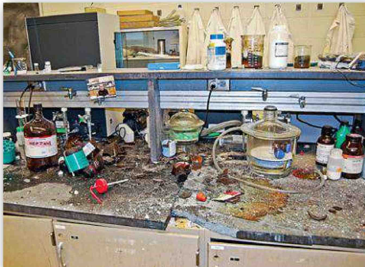
On Jan. 7, 2010, Texas Tech University (TTU) graduate student Preston Brown was working to synthesize and characterize an energetic material (nickel hydrazine perchlorate) when an explosion occurred. Brown lost three digits on his left hand, severely lacerated his right hand, perforated his left eye, scratched his right eye and had superficial cuts to the parts of his body that were exposed.
