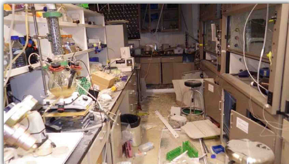
A powerful explosion at a University of Hawaii science lab was likely caused by a digital pressure gauge that shouldn't have been used around flammable gases (18/04/2016).
